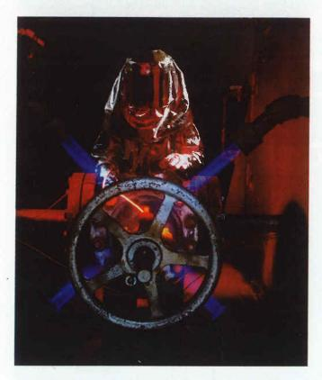
At the Garlock on site fire test facility, valves and sealing materials are functionally tested in the most extreme applications. 9000 EVSP Simplified meets these stringent fire test standards.
