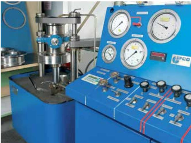
To ensure consistent high quality valves all components are subjected to stringent testing running in parallel with all stages of production.
