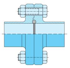
Aseptic flange connection in Off-Load design.
