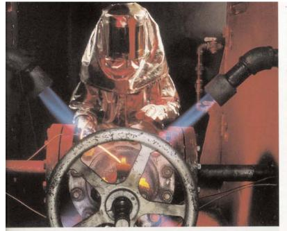
Style 1303 FEP has been successfully fire safe tested to API 589 standards at API 607 temperatures and pressures. In hot air weight loss tests, Style 1303 FEP experiences less weight loss than all other spool stock packings tested.
